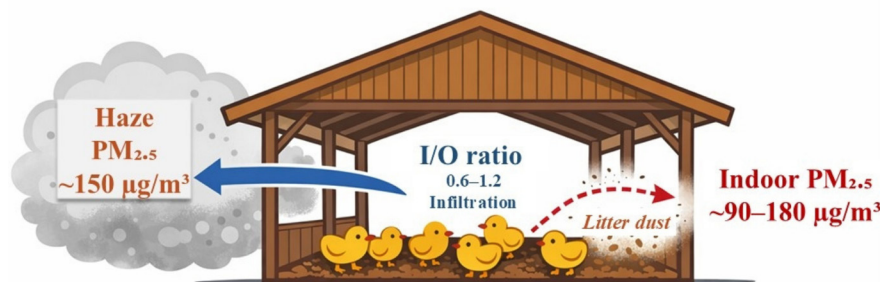
Figure 2. Schematic illustration of haze PM2.5 infiltration into an open-sided broiler house under naturally ventilated tropical conditions. Outdoor haze PM2.5 and indoor litter/feed dust jointly contribute to the estimated indoor PM2.5.
