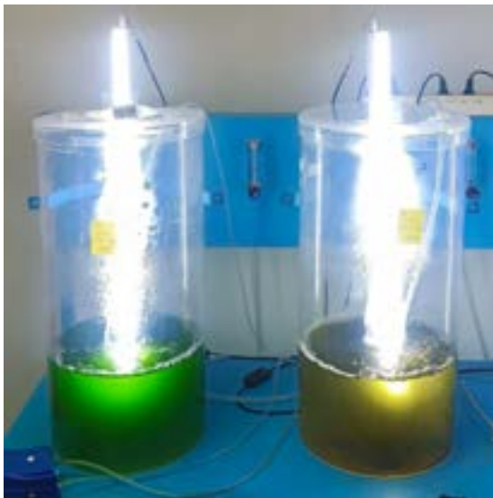
Gambar 1. (A) Bioreaktor vertical tubular reactor (B) Skema VTR
