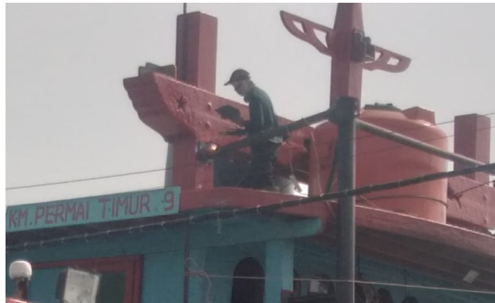
Figure 6 Workshop worker welding component (mast) at pier
