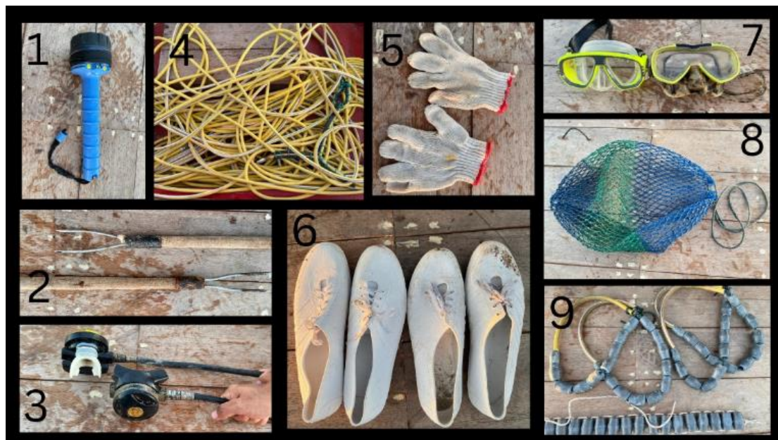
Gambar 4 (1) Senter; (2) Tombak; (3) Regulator; (4) Selang kompresor; (5) Sarung tangan; (6) Sepatu; (7) Fish mask; (8) Kantong jaring; (9) Timah
