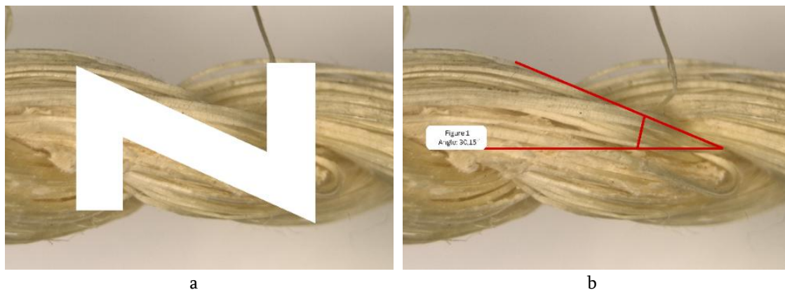
Figure 1 Pineapple fiber rope (a) Direction of S-twist; (b) Twist angle of pineapple fiber rope
