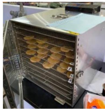
Figure 2. Arrangement of apple slices on trays inside the Wirastar FDH-10 food dehydrator
