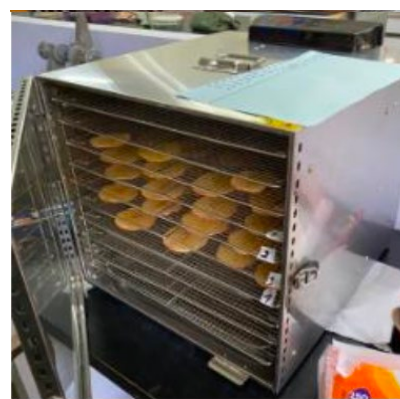
Figure 2. Arrangement of apple slices on trays inside the Wirastar FDH-10 food dehydrator
