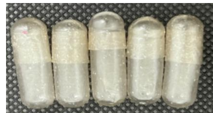
Figure 1. Hard capsule produced from mixture of konjac glucomannan and carrageenan
