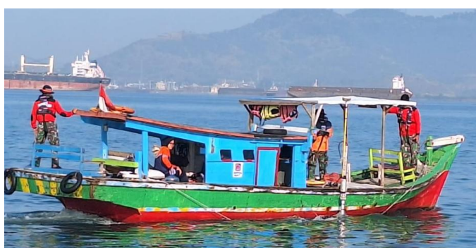
Figure 2. Sounding boat that served as the primary vessel for the hydrographic survey around Panjang Island. This vessel was equipped with a diesel engine and provided the necessary platform for mounting the SBES and RTK positioning systems.
