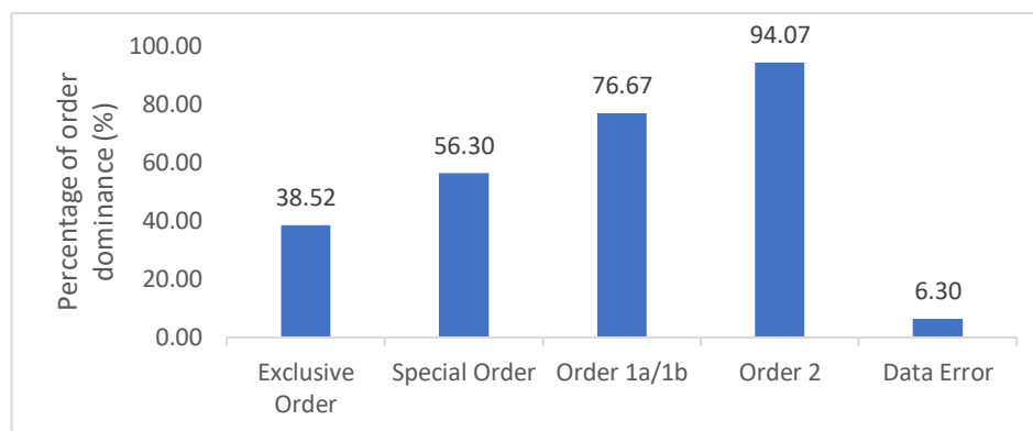
Figure 8. The quality of the bathymetric data according to IHO S-44 survey order standards. The chart shows that while 94.07% of the data meets Order 2 standards, only 38.52% reaches the high-precision Exclusive Order level required for the most demanding maritime applications.
