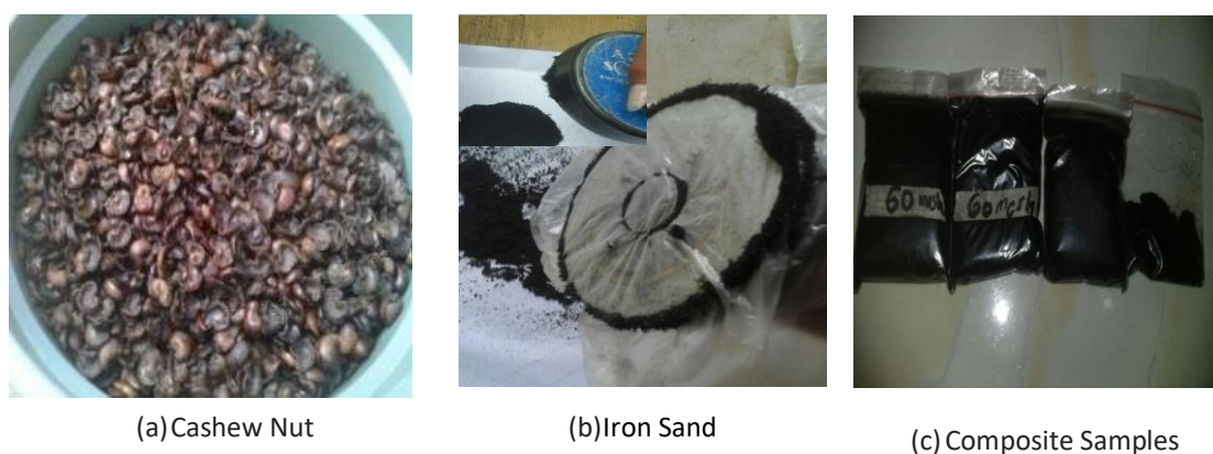
Figure 1. Preparation Sample Processes: (a) Raw Material of Cashew Nut; (b) Magnetic Extraction of Iron sand; and (c) Composite Samples.
