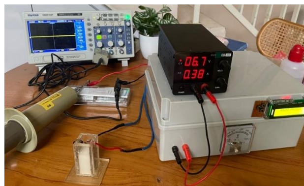
Figure 3. Photograph of the developed laboratory-scale PEF system and experimental setup used for electrical characterization and solid-food treatment. The setup consists of a high-voltage generator, a treatment chamber, a DC power supply, a digital oscilloscope, and a high-voltage probe
