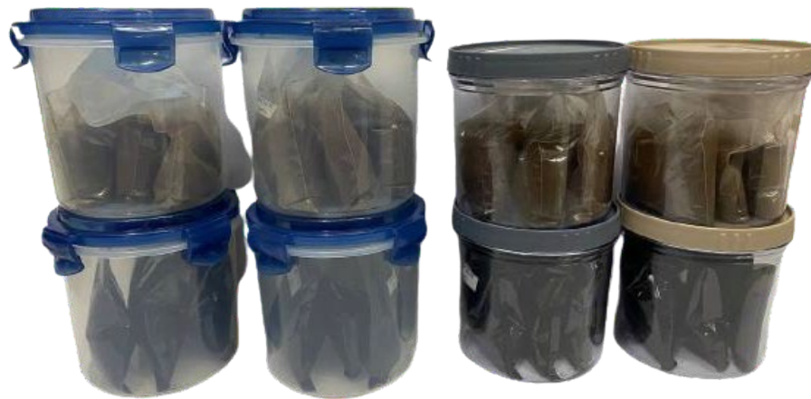
Figure 3. Airtight (left) and non-airtight containers (right) with transparent (top) and opaque packets (bottom).
