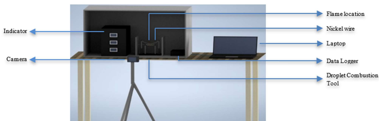
Figure 5. Droplet test combustion chamber.
