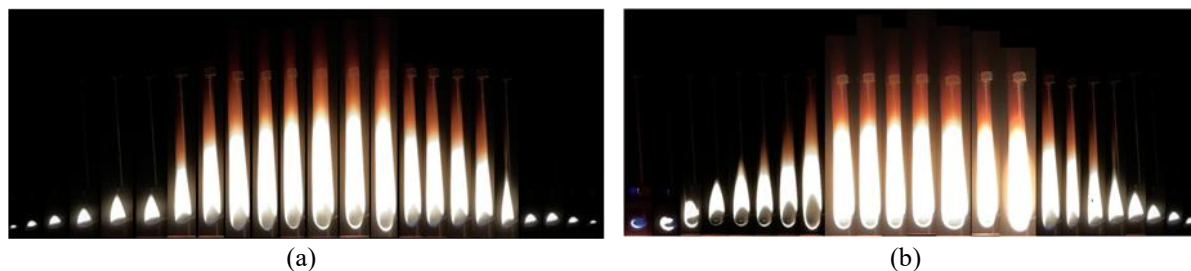
Figure 15. Visualization of Flame with composition (a) B100 and (b) B100+TiO 2 .
