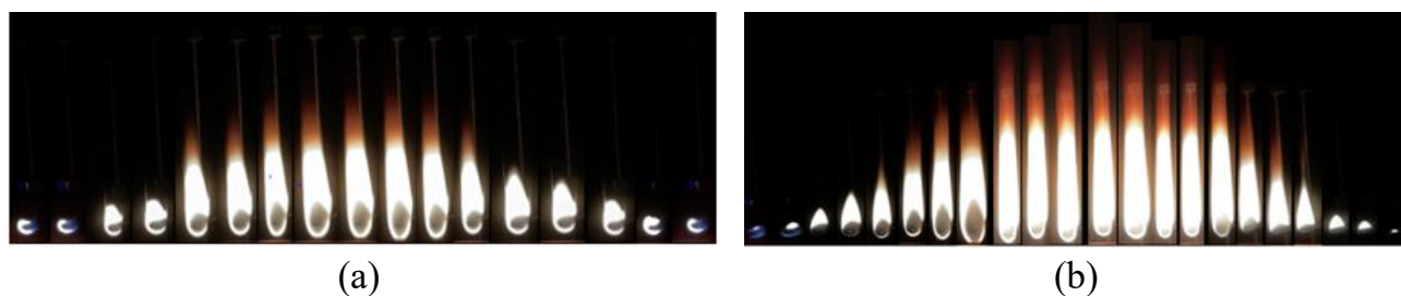
Figure 10. Flame Visualization with Compositions (a) B0 and (b) B0+ \text{TiO}_2 .
