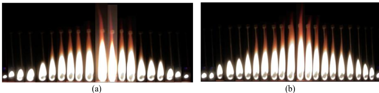
Figure 13. Visualization of Flame with composition (a) B30 and (b) B30+TiO 2 .
