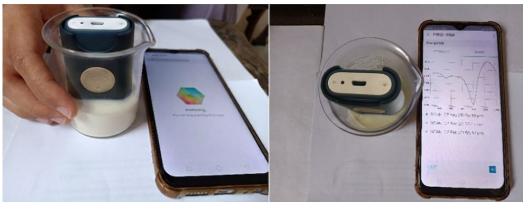
Figure 1. Acquisition of spectra data of milk sample using SCiO NIR device.
