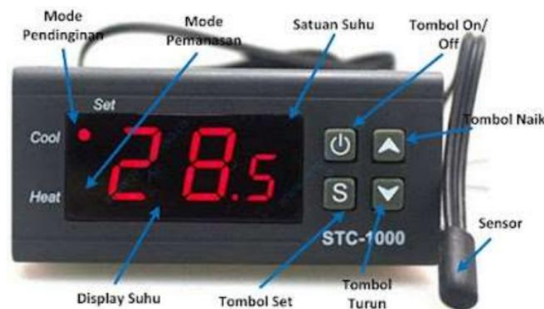
Figure 7. Parts of the STC-1000 thermostat (Simamora et al. 2023).
