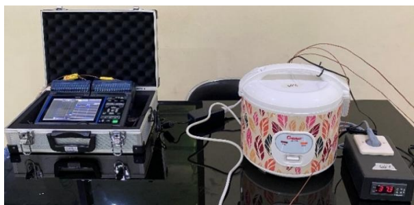
Figure 9. Temperature calibration circuit using a thermo recorder.
