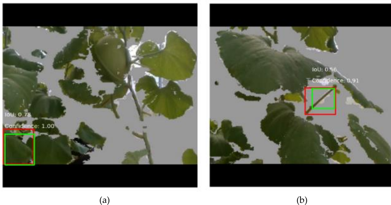
Figure 7. Objects that are successfully detected by the best model (a) leaf (b) branch of melon plant
