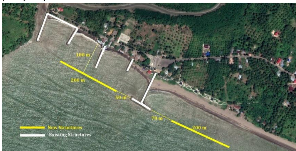
Figure 9. Proposed shore protection structure layout for Tugu Beach based on 2019 Google Earth imagery
