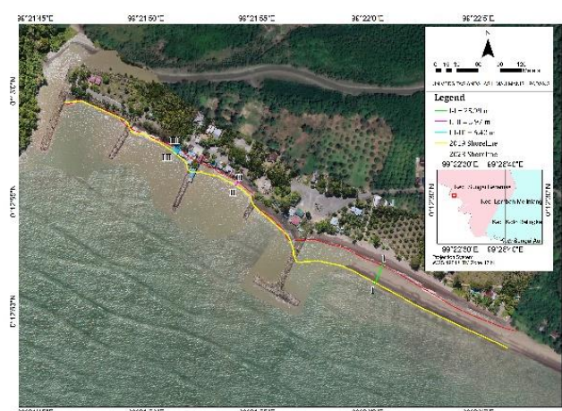
Figure 6. Shoreline Digitization: Comparison of shoreline positions derived from Google Satellite Imagery (2019) and Aerial Photography (2023)
