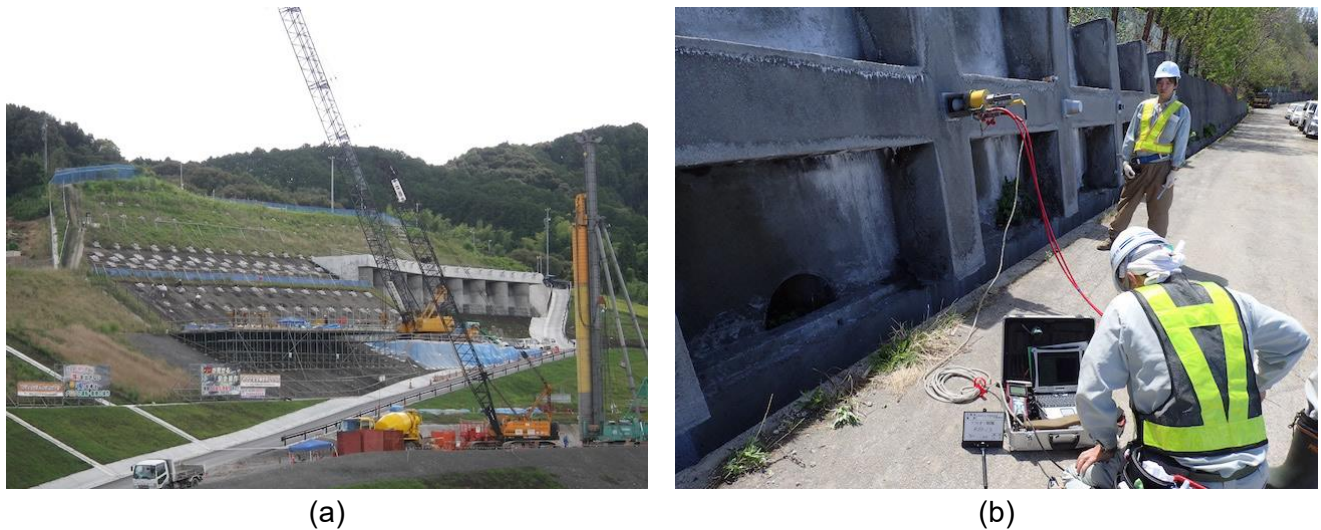
Figure 3. (a) Liftoff test with a center-hole jack, (b) Residual-stress survey using the SAAM system
