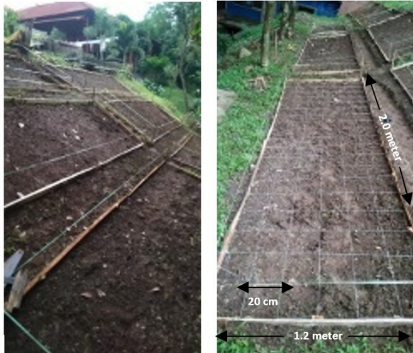
Figure 2. The experimental plots were conducted on a slope of 15-25%. Sample plot unit (OSPs) were constructed with modified dimensions of 2.0 m × 1.2 m, adjusted from the original 4.0 m × 1.2 m layout in campus area of Nusa Bangsa University. Those plots were adapted to the condition and limitations of the land.
