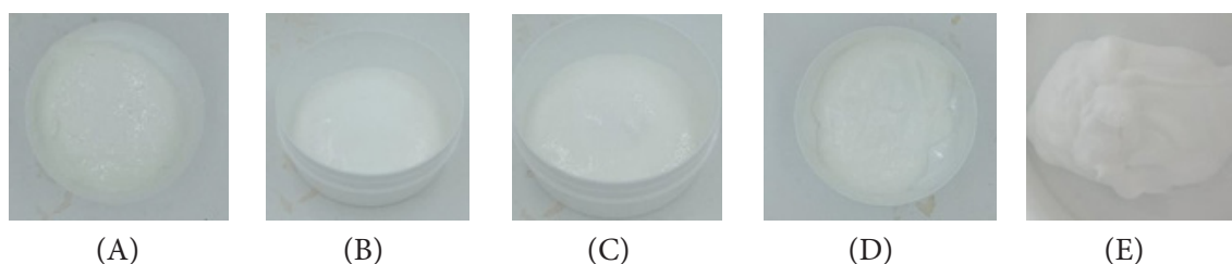
Figure 3 Body lotion appearance addition chitosan alginate nanoparticles (g); (A) 0, (B) 1, (C) 2, (D) 3, (E) commercial
