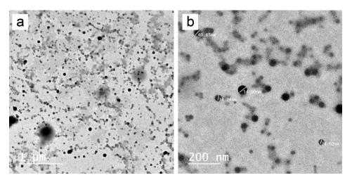
Figure 5. Transmission electron microscopy (TEM) of thymol oil nano emulsion (a-b) showed the morphological shape of nanoparticles (a) that appeared as a fine spherical particle distributed in the TEM field, and the average diameter of nanoparticles (b) is ranged from 24.02 to 54.0 nm
