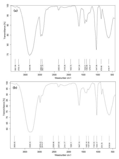
Figure 4. FT-IR spectra of cinnamon oil (a) at infrared wavelength 3350.96-619.71 cm<sup>-1</sup> and infrared wavelength of cinnamon nano-emulsion (b) was 3328.33-618.64 cm<sup>-1</sup>
