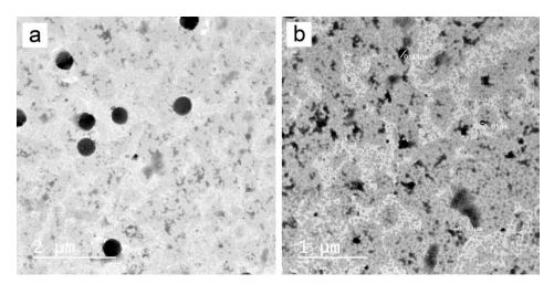
Figure 6. Transmission electron microscopy (TEM) of carvacrol oil nano-emulsion (a-b) revealed the nanoparticles of spherical shape scattered into the nano-emulsion (a), and the average size of nanoparticles is ranged from 0.03 to 0.13 µm as shown in (b).
