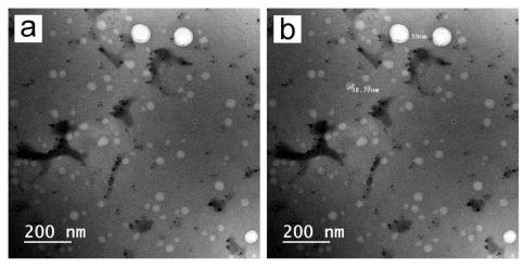
Figure 7. Transmission electron microscopy (TEM) of basil oil nano-emulsion (a-b) displayed the spherical and ovoid shape of NPs scattered in the field of TEM (a) with the average size is ranged from 38.72 to 65.59 nm (b).
