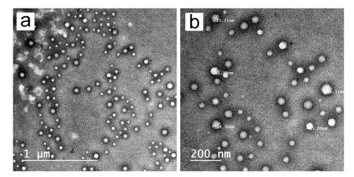
Figure 8. Transmission electron microscopy (TEM) of cinnamon oil nano-emulsion (a-b) presented very fine spherical NPs in shape and had a raised surface (a) besides the NPs size (b) is ranged from 53.21 to 54.30 nm in diameter.
