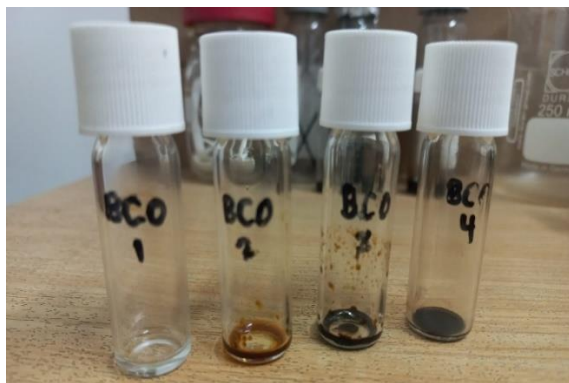
Gambar 9. Hasil fraksinasi biocrude oil (BCO) pirolisis sabun logam
