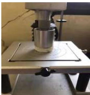
Figure 3. Cylindrical probe type 35 mm
