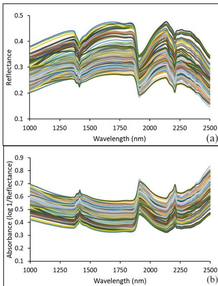
**Figure 2.** (a) Reflectance spectra and (b) absorbance spectra of NIR wavelengths from soil samples.
