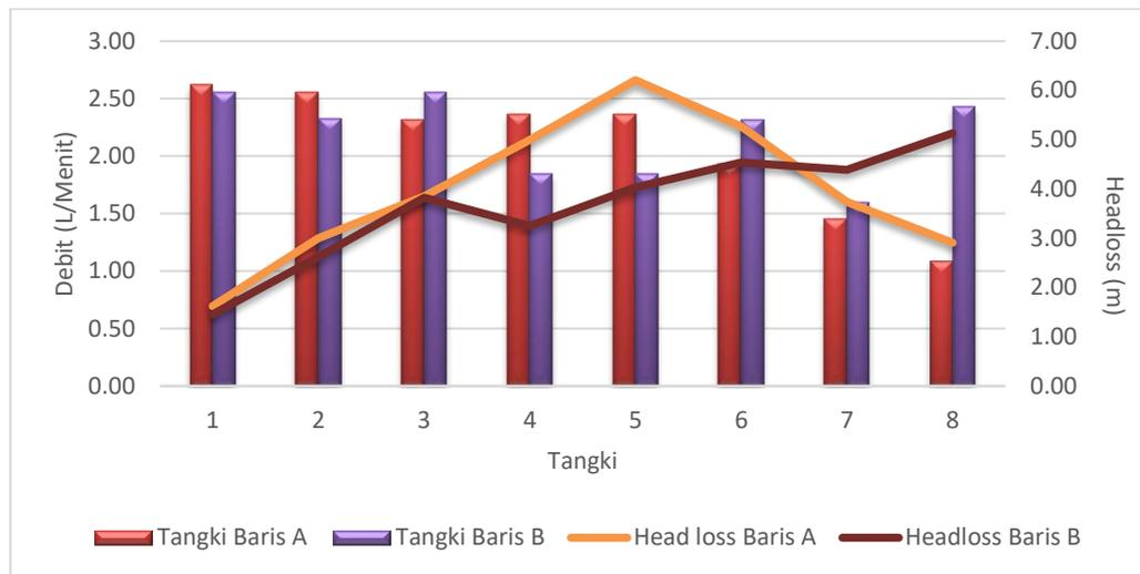
**Figure 3.** Initial Measurement of Discharge and Headloss.
