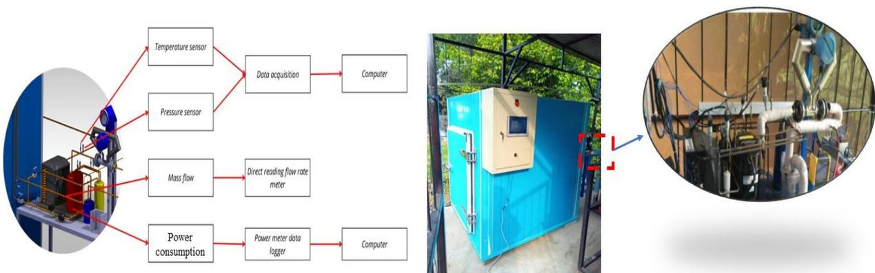
**Figure 3.** (a) Experimental setup for laboratory testing and (b) actual laboratory conditions.
