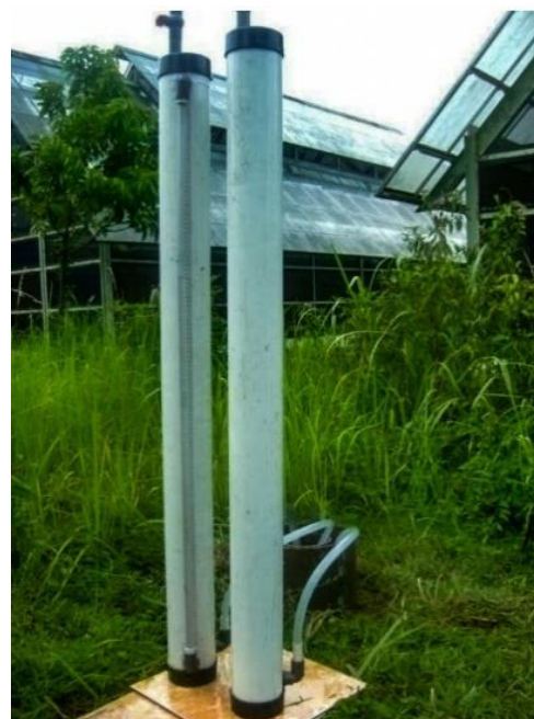
Figure 2. Mariote siphon developed to maintain a constant head in infiltration ring
