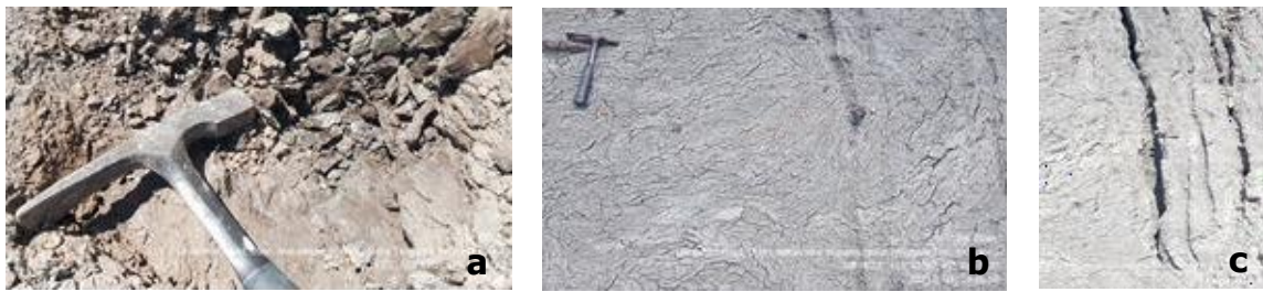
Figure 3. a. showing the mélange clay of the Bobonaro Complex with a scaly clay structure; b. mixed rock clay surface with flow structure influenced by rainwater and c. flow-type avalanche grooves.
