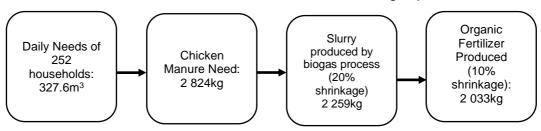
Figure 2 The process of chicken manure into biogas
