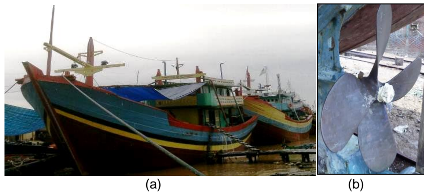
Figure 1 (a) Fisherman wood boats in a north Java Island port and (b) the propeller installed on the wood boats, made by SME in Tegal.
