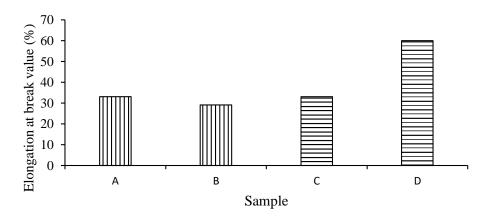
Figure 2 Elongation at break of bioplastic
