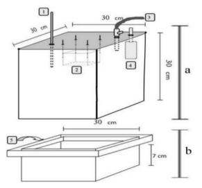
Figure 2 Design of chamber (a) and chamber base (b), including thermometer (1), mini fan (2), hose system (3), pressure compensation bag (4), and water reservoir (5)
