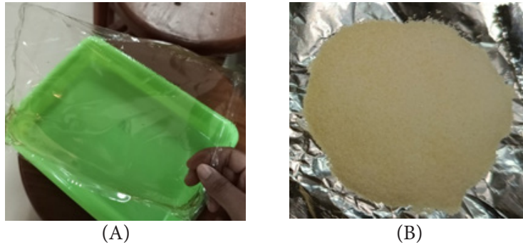
Figure 1 The image shows the appearance of pangasius skin gelatin (A) before grinding and (B) after grinding
