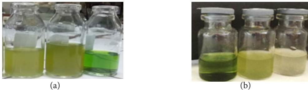
Figure 1 Sea grape extracts using maceration method (a) and MAE (b). From left to right, ethanol, distilled water:ethanol, and distilled water extract.
