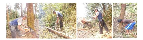
Figure 1 The difficult work postures at activities of (a) felling, (b) delimbing, (c) bucking, and (d) hauling.
