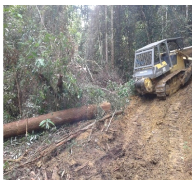
Figure 4 Skidding activity in the logging area and tilted damage on the residual stand due to timber skidding.
