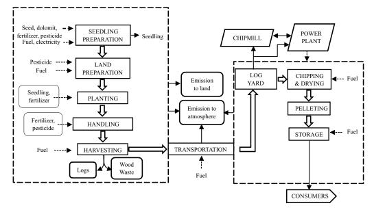
Figure 2 System boundary of wood pellet production.
