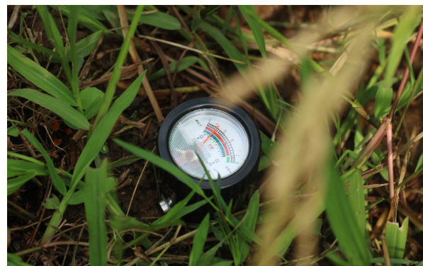
Figure 3 Device used by farmers to measure the soil pH showing acidic soil (pH 4.2).
