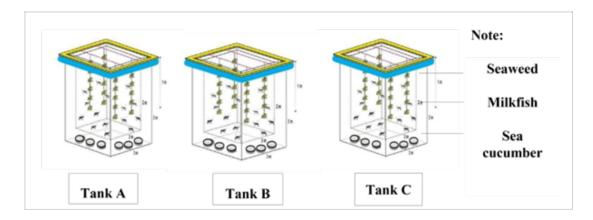
Figure 2. Rearing media design with sand sea cucumbers (H. scabra), milkfish (Chanos chanos), and seaweed (Euchema cotonnii) with IMTA system.
