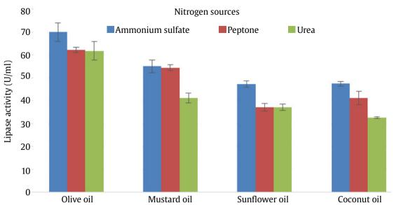
Figure 7. Lipase activity of *L. sphaericus* L49a produced after 20 hours cultivation in medium containing different nitrogen sources and vegetable oils
