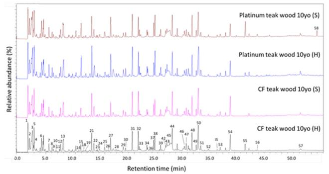
Figure 2. Py-GCMS pyrogram of 10 years-old Tectona grandis for fast-grown platinum and conventional teak wood. The Pyrolysis product peaks (1-58) are presented in Table 1, and n-eicosane for internal standard (IS)
