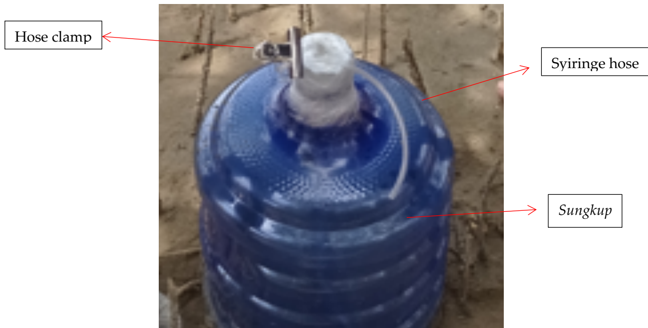
Figure 2. Sungkup (gas trap)
