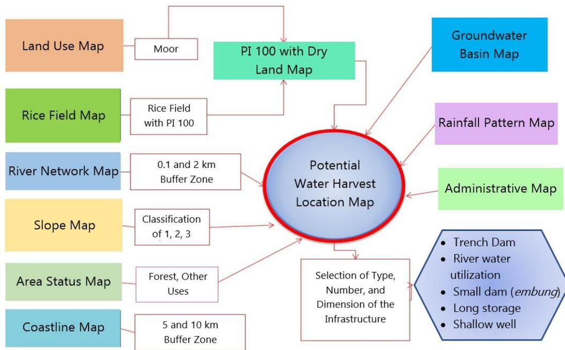
**Figure 1.** Diagram of the stages of determining the location and selecting the water harvesting infrastructure
