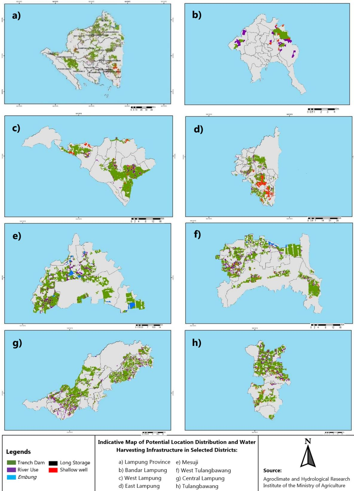
**Figure 3.** Indicative maps of potential location and type of water harvesting infrastructures in Lampung Province (a), and in (b) Bandar Lampung; (c) West Lampung; (d) East Lampung; (e) Mesuji; (f) West Tulangbawang; (g) Central Lampung; and (h) Tulangbawang
