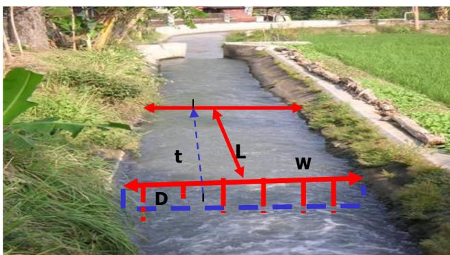
**Figure 2.** Design of flow discharge measurement in the field
