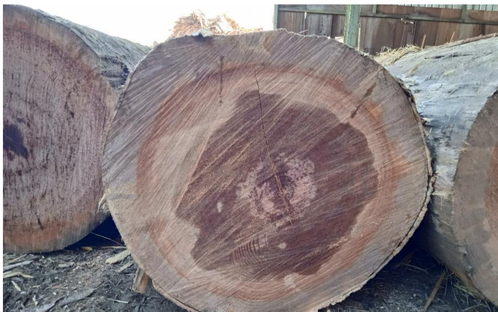
Figure 6 Keruing oil visible on the log.
