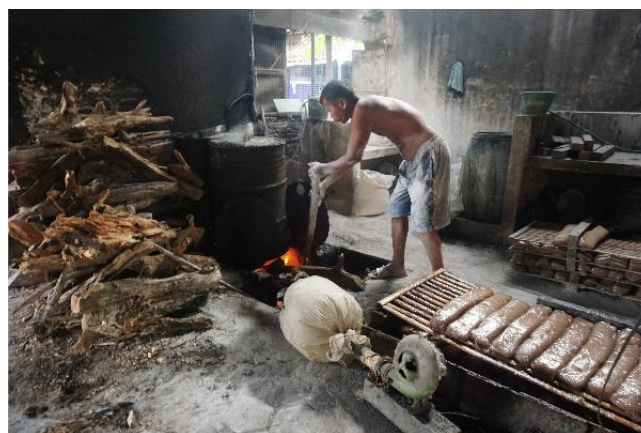
Figure 1 Cooking tapioca flour using a scrap iron drum.
