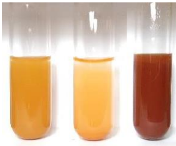
Figure 1 \text{Cu}_2\text{O} products with various types of reducing agents, sucrose (a), white sugar (b), and brown sugar (c).
