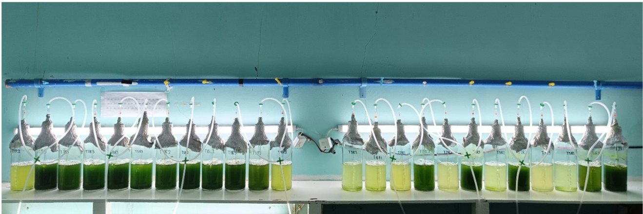
Figure 2. Experimental set-up. The glass bottles were enriched with different salinity concentrations ( \text{g L}^{-1} ) and AMPEP concentration in a nutrient medium
