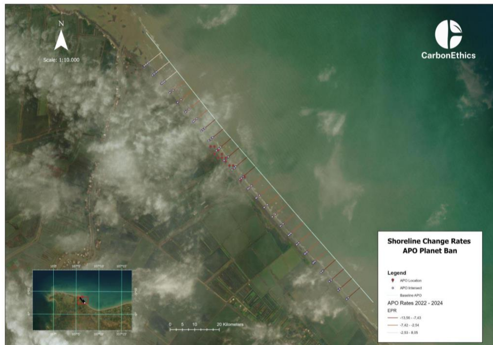
Figure 6. Spatial distribution of shoreline change rates around APO (waste-tire wave breakers) installation areas in Tanjung Pakis Village, Karawang Regency, West Java, Indonesia, based on DSAS End Point Rate (EPR) analysis for the 2022–2024 period
