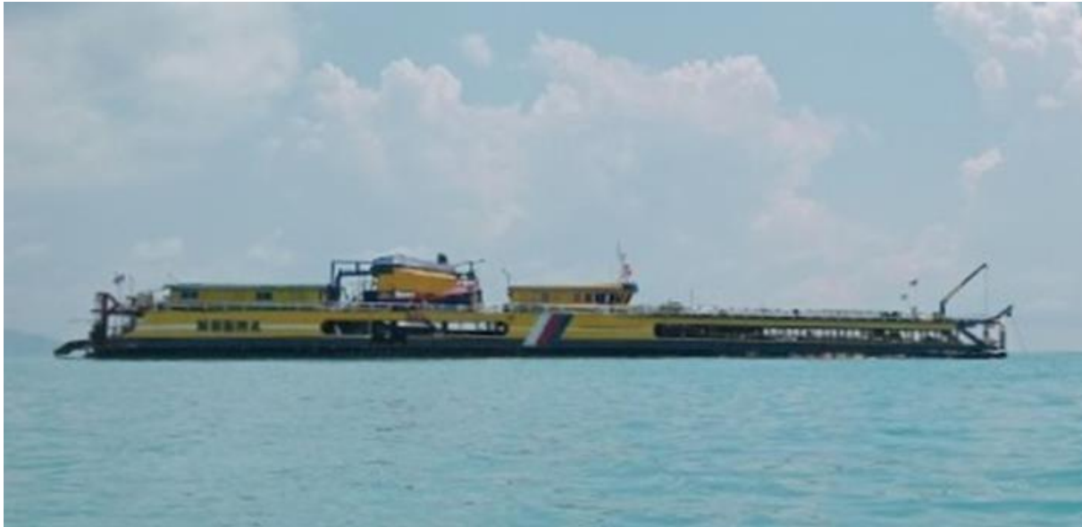
Figure 1. Dredgers operating in the coastal waters of the Northeastern Coast of Bangka Island dredge sand from the seabed, washing the material using a jigging system, and extracting the tin ore contained within
